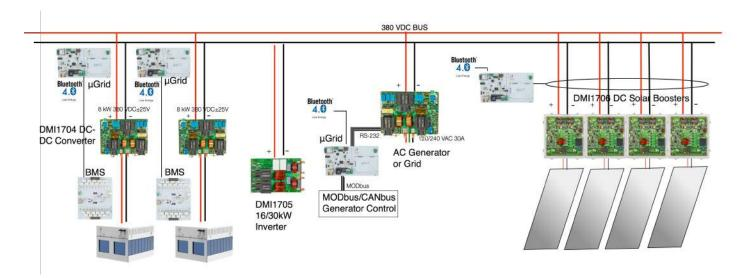
management. The  $\mu$ GridLink configures the BMS cards first and sends a request for battery voltages. Then, it makes a decision based on the health of the battery to allow charging or discharge of the battery.
