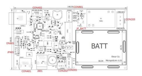
Switch's LED pins (CON201) are two outputs directly out of the microprocessor atsam3s at 3.3V level.
